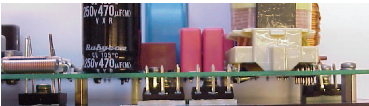
Pic. 27: Main electronic components on power board on heat sink
