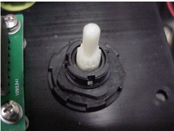
Pic. 14: UPPER part power circuit breaker
